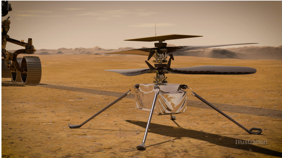
Figure 2: The Ingenuity drone with its helicopter rotors ready to take off, with the solar panel used to charge its battery on the very top. In the background you can see a part of the Perseverance rover. Credit: NASA/JPL-Caltech.
